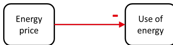
Figure 8. Components in a CLD – variable, link between variables, and sign (+/-) of one variables effect on another variable (in this case, as energy price goes up, use of energy goes down)
